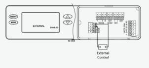
The Model A710 can be controlled with the Model A77 Control (included) or any external control that can provide a dry contact closure. When the Model A77 is used, the User Interface on the dehumidifier **MUST BE** set to "Remote". For all other external controls, the User Interface **MUST BE** set to "External". Refer to the quick start guide or installation manual for instructions on accessing the installer set-up menu.
